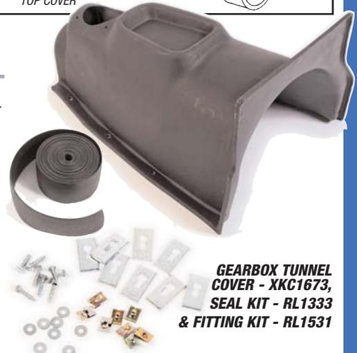
**GEARBOX TUNNEL COVER - XKC1673, SEAL KIT - RL1333 & FITTING KIT - RL1531**
