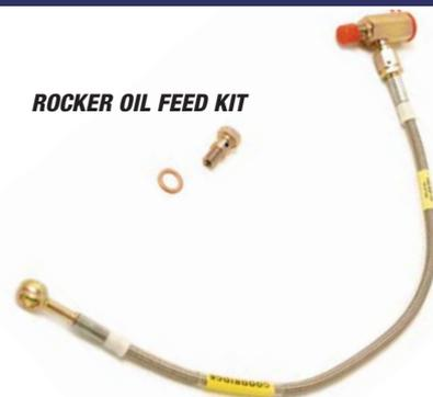
Excessive rocker shaft wear is a classic complaint about the Triumph push rod engines. The external rocker feed kit is an effective and easy to fit solution to the problem. It works by piping oil from a plug hole in the cylinder block main oil gallery up to the cylinder head, thereby maintaining a higher oil flow than standard. No drilling or tapping is required for installation. The kit is so good, it looks as though it should always have been there!
