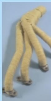
By wrapping your tubular manifold with Thermo-Tec insulating wrap you can overcome all these risk factors. Thermo-Tec keeps the heat within the manifold so the exhaust gases have a much higher velocity, this induces negative pressure (scavenging) which increases air intake flow, resulting in better performance & economy. It also reduces under bonnet noise.
