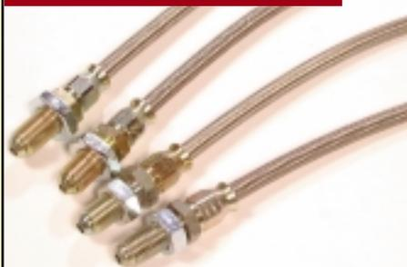
Replace those bulging rubber flexible hoses with these stainless steel braided hoses for firmer brake pedal pressure. Kits include front & rear flexible brake hoses.
