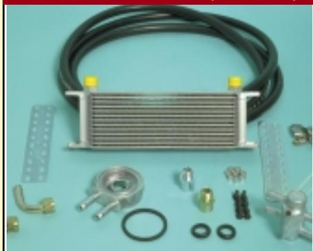
If high oil temperatures are a problem, for example when towing, the V8 engine will benefit from the fitting of an oil cooler. We recommend fitting a thermostat at the same time, to avoid overcooling.
