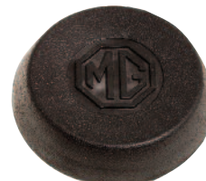
BOSS, STEERING WHEEL (HORN PUSH TYPE) - BHA5043
