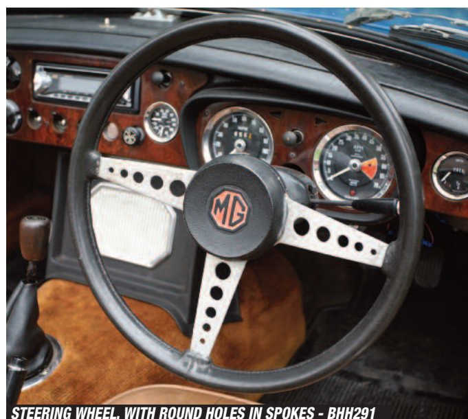
STEERING WHEEL, WITH ROUND HOLES IN SPOKES - BHH291
