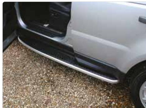
VPLSP0040 Side Steps Side steps with thermo plastic elastomer side step top and brushed aluminium side trim. Pair.
