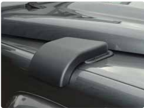
Snow Cows Manufactured from ABS plastic these cowl will help prevent snow, mud and leaves from entering the heater intake and reducing the Defender heater performance. Fitting a cowl will reduce moisture build-up in the intake system which can happen if debris collects in the one-way valve. The cowl fits over the existing grille and follows the profile of the Defender's wing. DA1270 Left hand drive DA1271 Right hand drive
