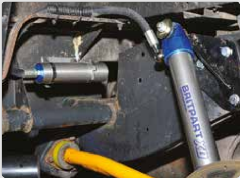
DA6323XD Front shock absorber turrets for use with the Britpart XD Remote Reservoir Shock Absorbers
