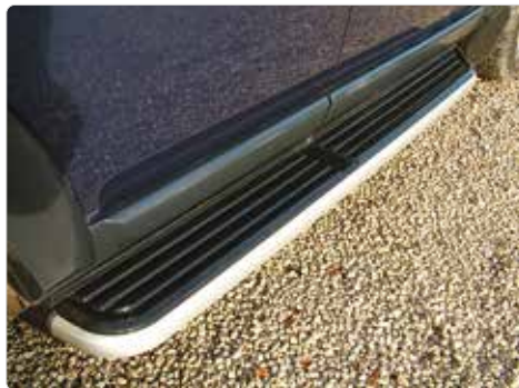
VPLAP0035 Side Steps Discovery 3/Discovery 4 Polypropylene side step top & brushed aluminium side Pair
