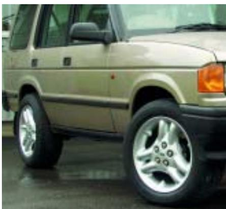
**18" TRIPLE SPORTS ALLOYS FITTED TO SERIES 1 DISCOVERY (APRIL '94 ON, 300 SERIES) USING HUB ADAPTOR KIT.**
