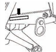
1. Stamped on the RH side of the chassis towards the rear of the front lashing eye.
