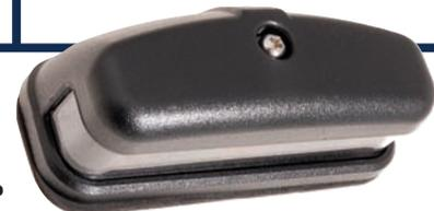
**REAR NUMBER PLATE LAMP ASSEMBLY - XFC100550LEDP1**
