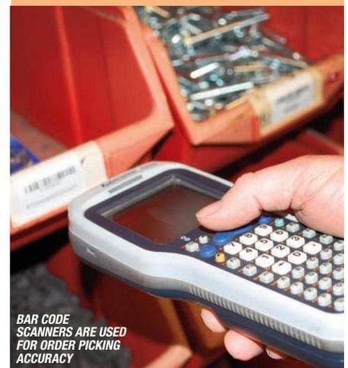
BAR CODE SCANNERS ARE USED FOR ORDER PICKING ACCURACY
