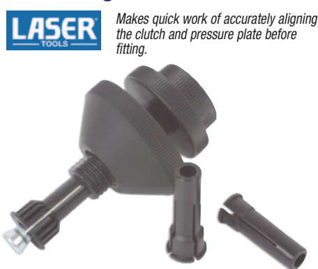
Clutch Alignment Tool Universal Laser RX1702 Fits most vehicles up to 5 tons except vehicles with double plate clutches. Body manufactured from ABS with brass screw and supplied with three collets. A full instruction leaflet is included.
