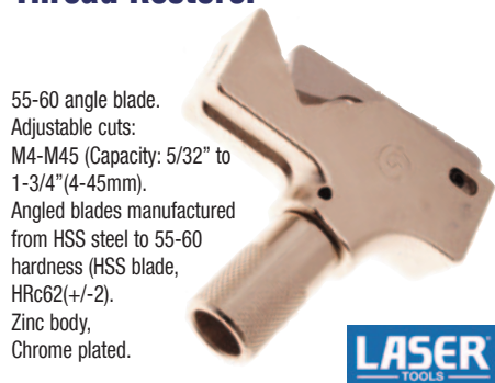
Adjustable Thread Restorer M4 to M45 Laser RX1969
