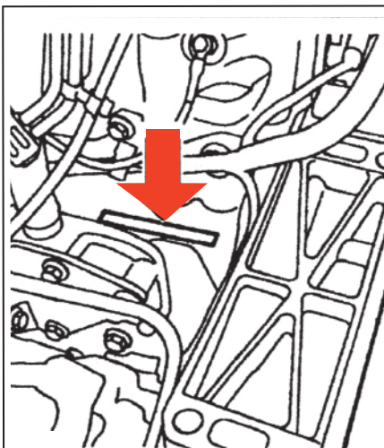
THE 300TDI ENGINE NUMBER IS STAMPED ON THE CYLINDER BLOCK ON THE RH SIDE OF THE ENGINE ABOVE THE CAMSHAFT FRONT COVER PLATE.
