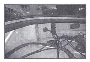
Route long part of harness through grommet on left hand side just above car main harness grommet. You will need to make a hole in original grommet. 10 Route harness along side main harness on left hand side, down 'B' post and along sill.
