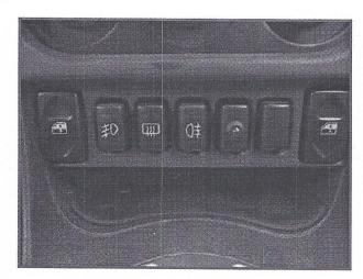
1 4 Drill a 8mm hole in a spare switch blank. Alternatively, if you have an early car, drill a hole in the centre of the switch mount. Fit lamp and connect wires (see picture which shows how unit comes apart for fitting).
