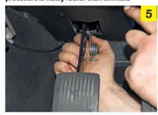
Next, ease the new spring into the bushes in the pedal and bracket. The trim may need to be pushed upwards to make this easier.
