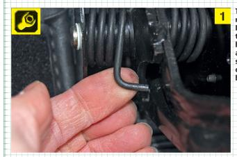
There are two throttle return springs on the Defender pedal. With this mod, the righthand spring is left alone. The left-hand spring must be levered out of the hole at the back of the pedal.
