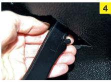
Disconnect the clutch return spring, then fit the three nylon bushes to the pedal and pedal box. The horseshoe-shaped bush fits into the pedal as shown here. The other two bushes have to be fitted by feel into holes in the clutch pedal bracket. The positions are obvious and the procedure is fiddly rather than difficult.
