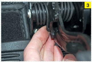
Clean up any rough edges with emery paper and touch up any scratches with black paint. Push the spring fully home.
