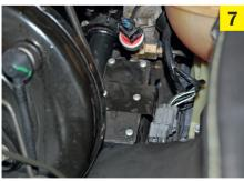
The clutch master pushrod-to-trunnion nut must be replaced and fully tightened. The job is finished by cleaning up and refitting the pedal box lid and fitting a new gasket if the old one is damaged. In this case, the gasket was fine and was re-used. It pays to go carefully here, as the gasket isn't cheap. Don't forget to reconnect the expansion chamber hose. Then it's just a matter of replacing the bonnet.
