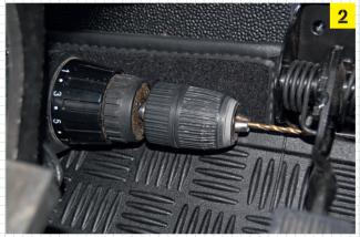
The new hole should be in the raised section of the pedal, quite close to the back. The centre of the hole is about 11mm into the raised section. measured horizontally from the cabin side of the pedal. Obviously, a sensible amount of metal must be left around the spring, so don't drill too close to the edge. Lightly centre-punching first helps with the drilling.
