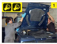
Ideally, the bonnet should be removed entirely to improve access to the top of the pedal box in the engine compartment. It simply needs to be raised to the upright position and then carefully lifted off. Two people should do this to avoid damage to the bonnet or wings.
