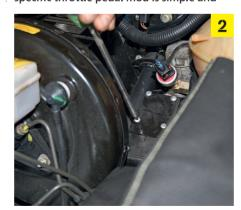
You should make sure that the engine is cool, then disconnect the pipe from the cooling system expansion tank to give you easier access to the screws that secure the top of the pedal box. Remove these screws and then lift off the top of the pedal box.
