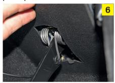
The new spring is now in position. Adding a little grease to the nylon bushes will help to make the pedal operation smoother.
