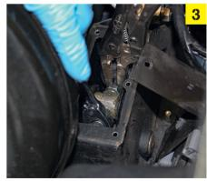
Get a mate to hold down the clutch pedal while you undo the nut securing the master cylinder pushrod to the clutch pedal trunnion. Hold with a suitable adjustable wrench while the nut is undone. The nut should be removed completely to allow full movement.
