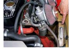
Check the VIN plate just behind the front left-hand shock absorber. If it's missing, then it may fail a UK MoT test. Performance air filters, a tubular steel exhaust manifold, and an alloy rocker cover are typical deviations from original specification.
