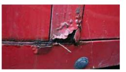
would not be great enough to warrant a lot being spent on it. Indeed, some examples ended up with more patchwork in the floor than original floor. Patches on patches not only weaken, but speed up future corrosion of structural panels.
