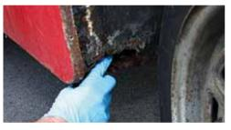
The box section in front of the toe board has completely rusted away, allowing even more water to penetrate. The sill closing plate is also allowing water into the sill cavity.
