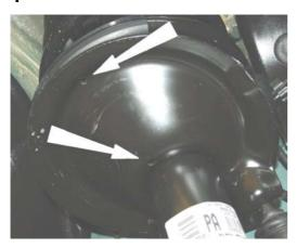
5. Referring to illustration 2a & 2b, position tyre protector to under side of spring damper cup, rotate protector until the stop on the protector contacts the spring end location on the damper. The 2 holes in the protector should now be in line with the holes in the damper.
