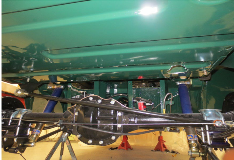
Panhard Rod Installed, on full droop
