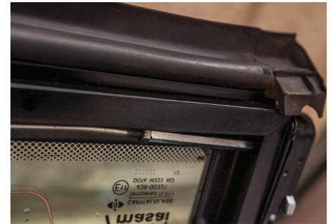
27. When the catches lock and unlock easily, refit the internal covers. Once covered, you won't be able to fettle with the rods any longer.
