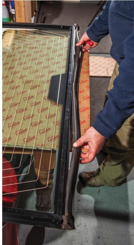
16. To refit the seal, tuck in either end, then the middle. Then, half the distance and tuck that in. Repeat until all is secured.
