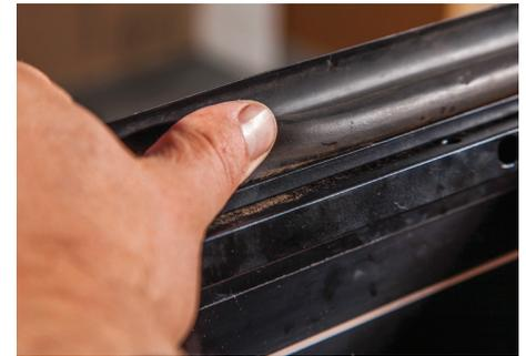
17. To check it is fitted correctly, carefully lift up the edge, checking along the length for bulbous areas that haven't been tucked into the retainer.
