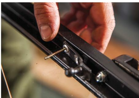
20. Finally, set about refitting the gas strut mounts using the rivets provided. The tailgate is now ready to refit onto the vehicle.
