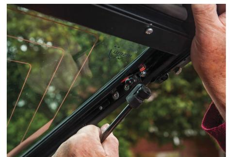
30. Set about refitting the gas struts (new units are recommended), the internal plastic lock cover and, last but not least, the wiper arm.
