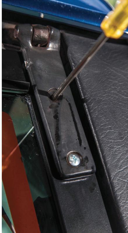
24. Finally, whilst keeping the top screwdriver in place, fit the lower mounting screw. You should then be able to remove the top screwdriver.
