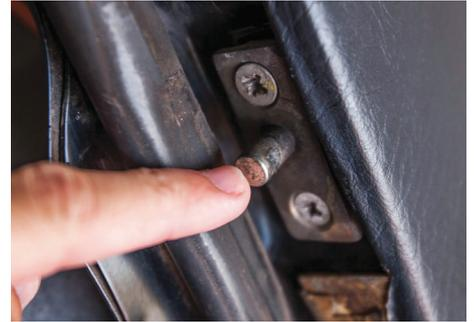
25. The catch plates on the body are adjustable, and the pegs offset. The plate may need turning around to get the peg in the right place for the new tailgate.
