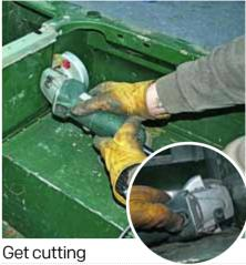
Using a 1mm cutting disc, cut along your line – straight down first, positioning the grinder's spark guard to stop you cutting too deep into the wheel box (inset). Do vertical cuts first, then horizontal. Keep cuts inside marked line. Work from rear side of bulkhead.
