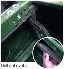
Drill out all the rivets in the top capping of the bulkhead panel then remove the two reinforcing sections, slotted underneath each side, using some water pump pliers. There may be some seam sealer in place on later models holding the sections in place.
