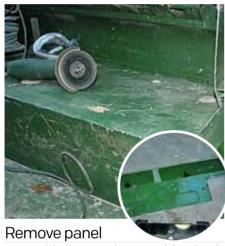
Finish by cutting into the support rib from the cab side of the bulkhead. The bulk of the unwanted panel can then be lifted out. Be careful of sharp edges at this point. Jack brackets may need to be removed first if you have them mounted to the front of the panel
