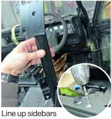
Drill out the rivet in front of the spigot nearest to where the bulkhead was (inset). Drill this out to 11mm. Position the left-hand sidebar upside-down on top of the 11mm hole on the right-hand side capping and mark the holes, then repeat with the other side.
