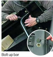
Before securing main brace bar to the side support brackets, use a 90° spike tool (inset) to remove plastic dust caps from mounting positions on floorpan. Attach loosely to one sidebar support (both if you can) to allow as much movement as possible.
