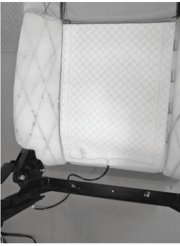
Undo the joining strip starting from one end at the rear bottom of the seat back, there may be 2 strings under the back of the seat cover that need undoing as well. Roll up the seat cover until you get to the bar fitting approximately two thirds of the way up.
