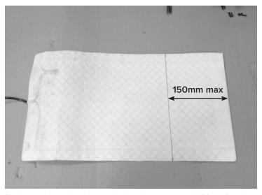
The heat pad may be shortened in length a maximum of 150mm from the end away from the cable.
