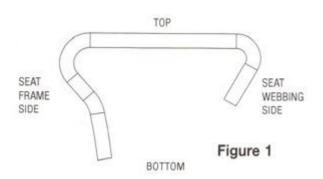
2. Start at the rear of the seat frame. Insert the two rods into the rear strap loops of the seat web assembly and attach the hook onto it as shown.
