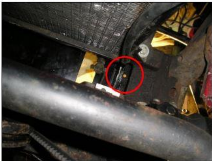
Fig 3: Fixing hole in chassis leg flange
